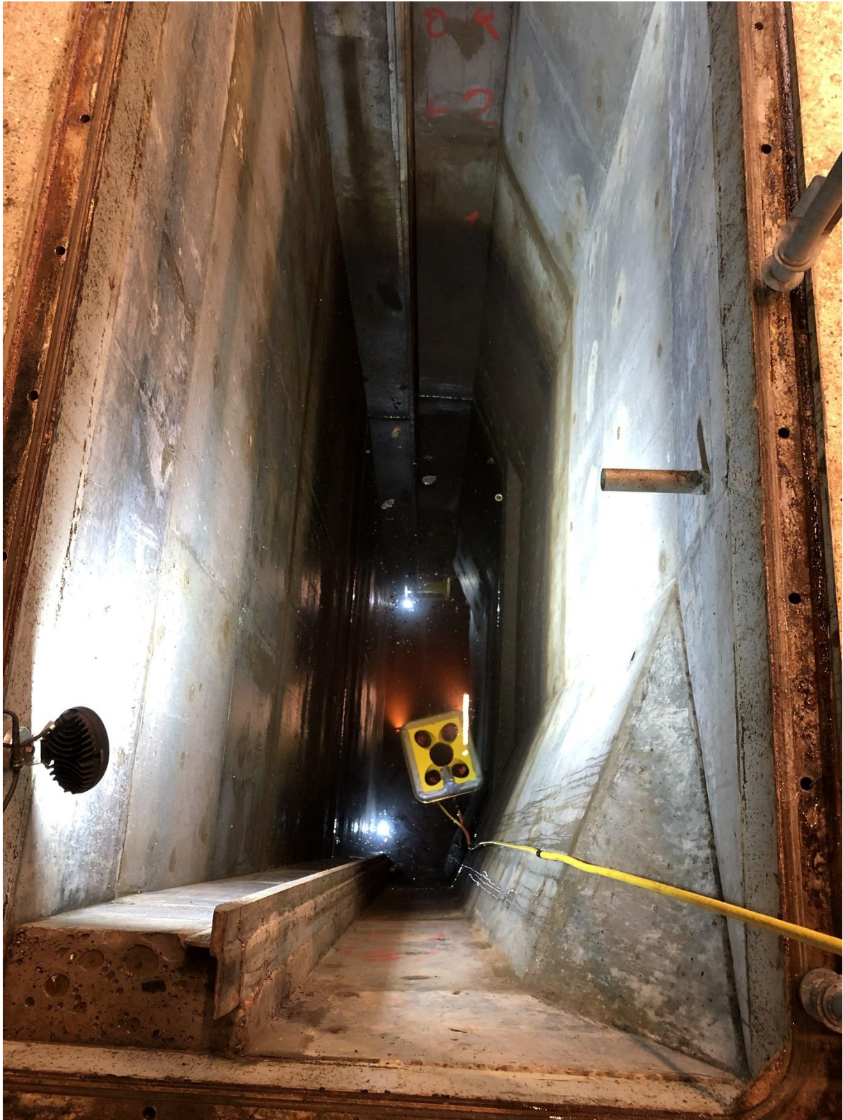
Figure 5. The entrance was narrow, but since the ROV can maneuver with 360 degrees of freedom, it was not difficult to dive down into the tunnel.
