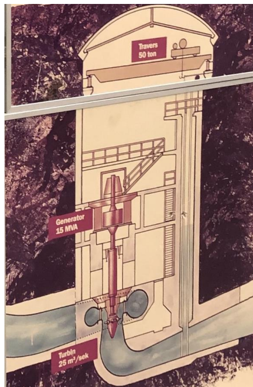
Figure 1. The ROV was lowered into the shaft seen to the right of the enerator and turbine.
